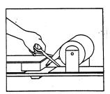
Feed the paper into the printer. Hold with one hand while pressing "PAPER FEED" button. Do not force the paper. The paper will advance slowly.
