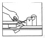
Replace the paper. Place the roll on the spindle. Reposition the spindle on the paper holder. Advance the paper and cut a straight edge; shiny side up.
